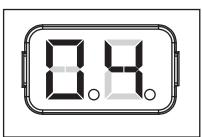
"0.4": During the system learning procedure, the control panel will automatically detect the current consumption from each motor, indicate the resistance level of the gate whiling the motor operation. If this reading increase instantly or stay in high reading, please check if any object in between of the gate moving area, and contact your installer for inspection.
