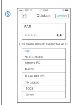
Select the Wi-Fi network for H210 and input the password, tap *Configure*. After hearing *success* from the device, you **NEED** to close the app and switch Wi-Fi network of your iPhone to the one which H210 is connected.
