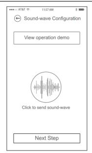
Keep the speaker of your phone close enough to the MIC of H210, click the sound wave icon to send sound wave, you can send it for many times until hear the voice "Receive network configuration", which means the device has joined the network.
