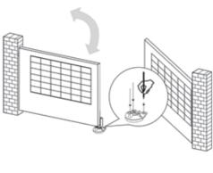
3). The gap between the bottom of electric latch and the stopper should be less than 7mm.
